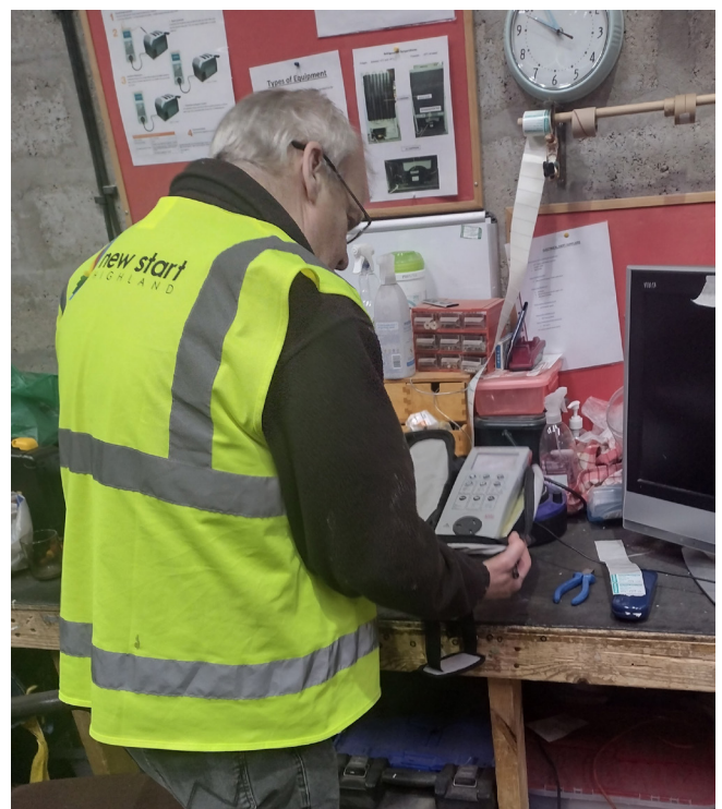
PAT Testing equipment
